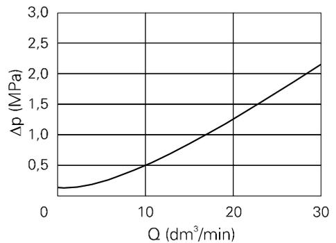
$\Delta p = f(Q)$  - pressure drop at check valve in relation to flow rate
