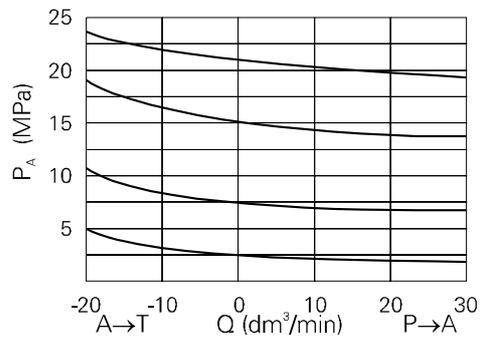
$P_A = f(Q)$  - output pressure in relation to flow rate
