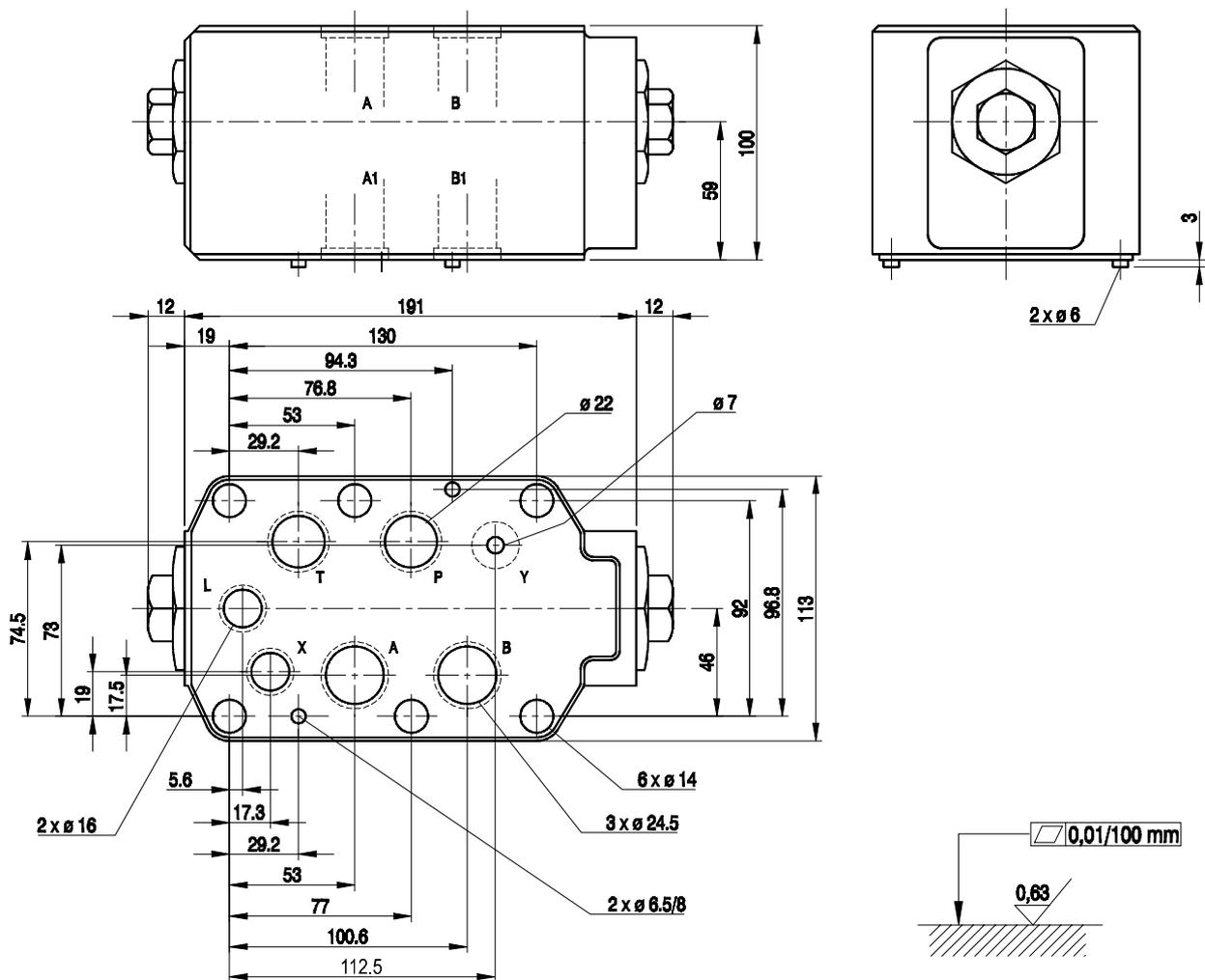
Admissible surface roughness and flatness deviation for a subplate face.
